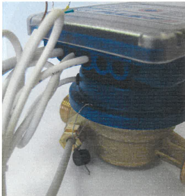
Pict. 6, Installation seal which assure a connection of one temperature sensor with the body of meter
