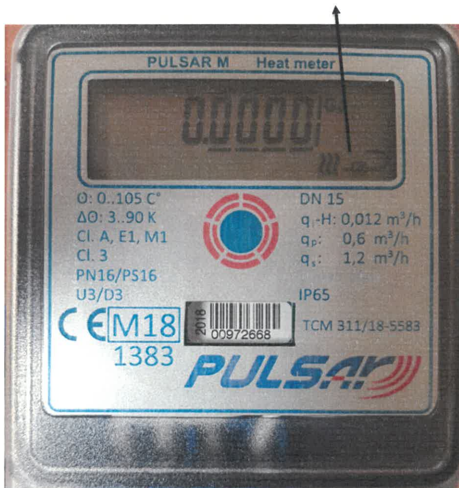
Pict. 1, inscription on Pulsar M heat meter (unit of measurement GJ, number of EU Certificate, main metrological label, other important information)
